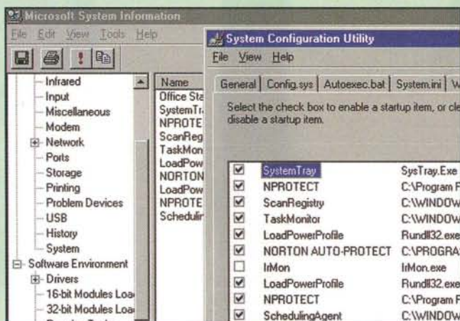
Windows 98's System Information utility has a configuration application that lets you change start-up features.
